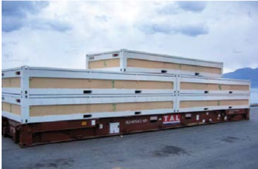
FLAT PACK containers ready for shipping in ship containers (flat rack) for distant locations
