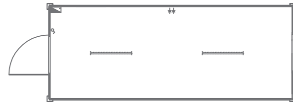
▲ P1 - 0001 storage container 6,0 x 2,4 m thermoisolated, door, finished el. cables, fuses, sockets, 2 ceiling lights, PVC floor
